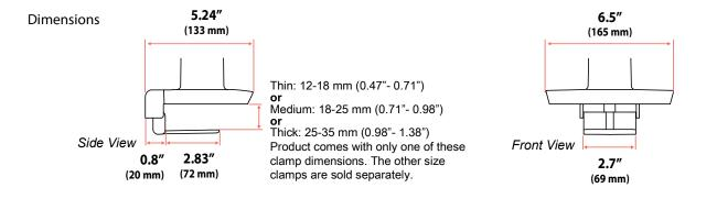
© 2020 Ergotron, Inc. rev. 01/30/2023 DIM-lowprofiletopclampkit Content is subject to change without notification
