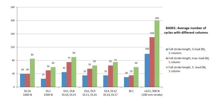
The graphic above shows average values. The measurements are made with control box CBD6S 300 W under the following conditions:
